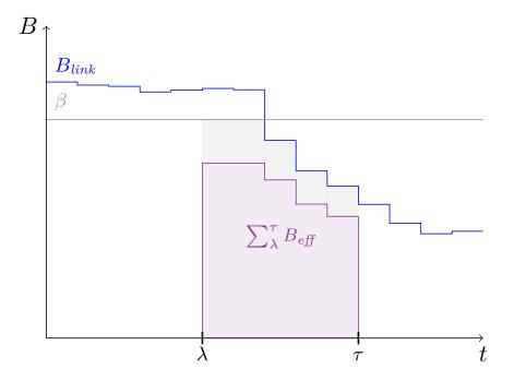
Figure 4.8: In addition to limiting the effective bandwidth by taking into account by the available bandwidth of the data producer  $\beta$ , an error margin is added, indicated by the gray area ( $\alpha = 0.8$ ):  $B_{eff} = \alpha \min(\beta, B_{link})$
