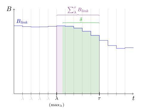
Figure 4.6: Data transmission in discrete quantities  $(\sum B_{link})$
