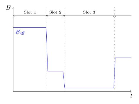
Figure 5.7: Slots with designated byte rates
